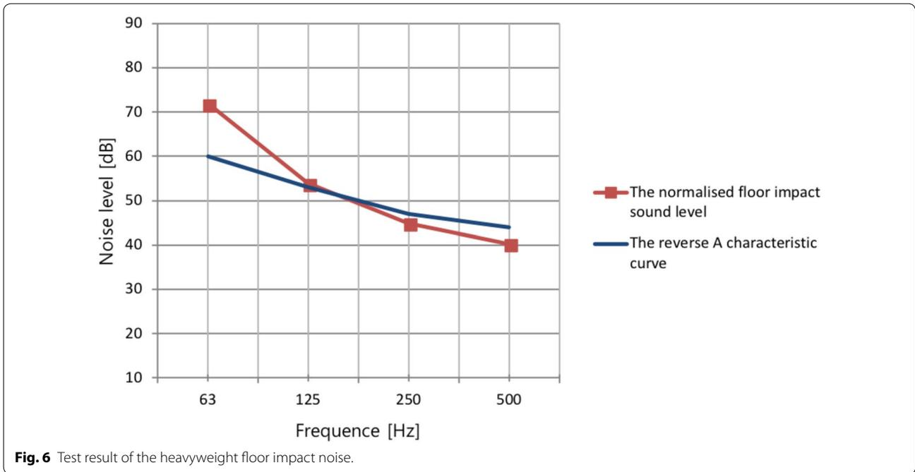
Fig. 6 Test result of the heavyweight floor impact noise.
