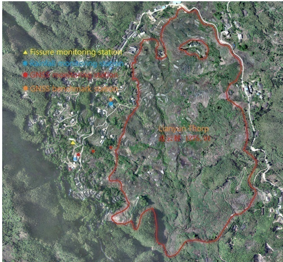
Fig. 10 Schematic layout of landslide monitoring locations
