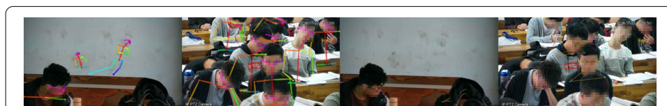
Fig. 5 Comparison of the pose estimation results. The pose estimation results of our method (right two images) and OpenPose method (left two images). OpenPose mistakenly identified wall patterns as human bodies, and the human pose estimation accuracy was poor. SE-HRNet yields significant improvements over OpenPose, reducing the human-body-object-detected error rate and increasing the accuracy of estimate key points
