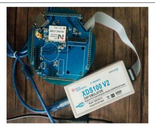
Fig. 6 The designed hardware for GPS/INS integration
