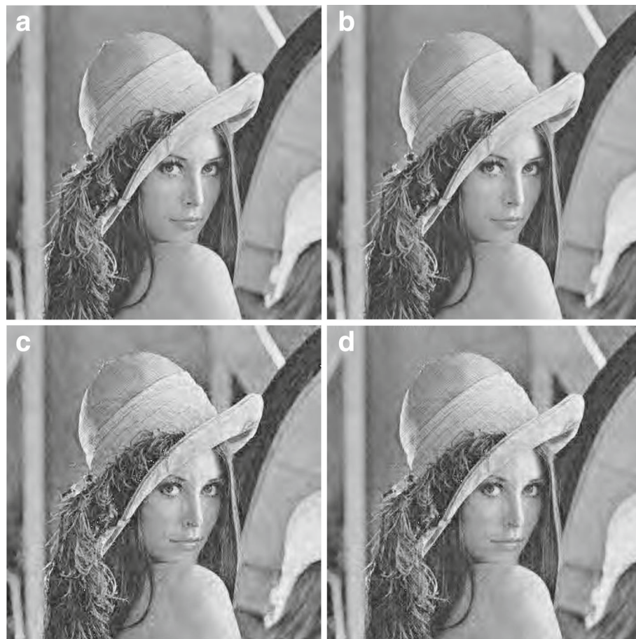
Fig. 6 Comparison of reconstructed images of “Lena” by the proposed predictive side decoding and the conventional side decoding: a the conventional 2-description side decoding (PSNR = 28.31 dB) versus b the proposed predictive 2-description side decoding (PSNR = 29.69 dB) at the same total bit rate of 0.537 bpp; c the conventional 1-description side decoding (PSNR = 26.43 dB) versus d the proposed predictive 1-description side decoding (PSNR = 27.68 dB) at the same total bit rate of 1.012 bpp
