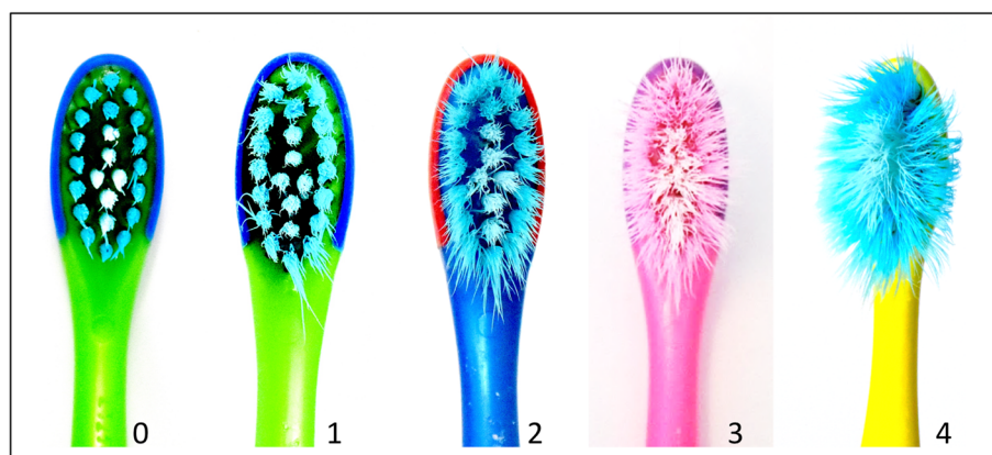
Fig. 1 Brush wear scores proposed by Conforti et al. [9, 14] The above images were not original pictures from the references
