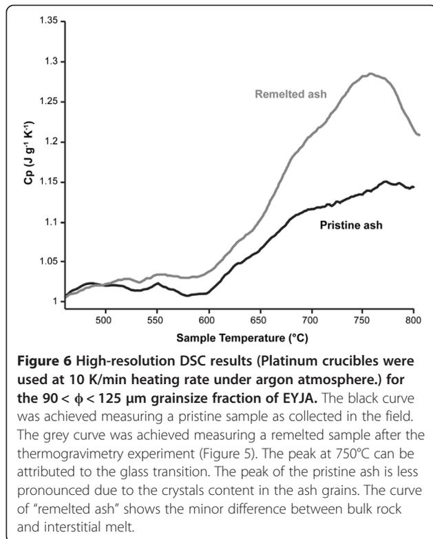
samples and not in the composition alone. The glass transition peak is less pronounced than for pure glasses; we relate this to the presence of crystals in the glass and a distribution of iron in different oxidation states (Kremers et al. 2012).
