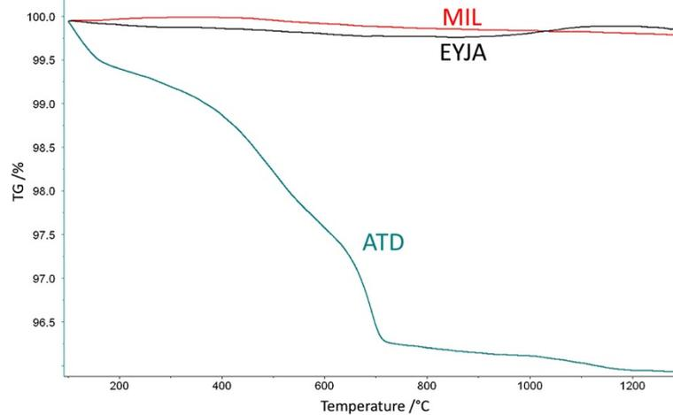
**Figure 4** Results of thermogravimetry analysis (Pt crucibles were used at 10 K/min heating rate under argon atmosphere.) for the  $90 < \varphi < 125 \mu\text{m}$  grainsize fraction. EYJA and MIL samples show a fairly similar behaviour whereas ATD shows a significant weight loss (4 wt.%) that can be attributed to decomposition reactions, most likely of  $\text{H}_2\text{O}$ -bearing phases.
