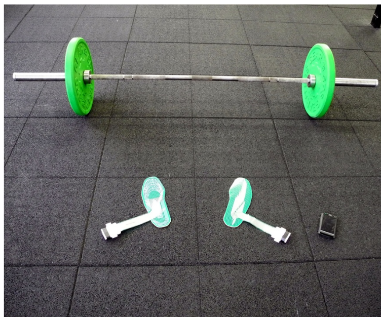
Figure 3 Study Equipment. Barbell with weights (40 kg); two sensor systems on plywood for left and right foot; smart phone controlling sensor systems and displaying data.
