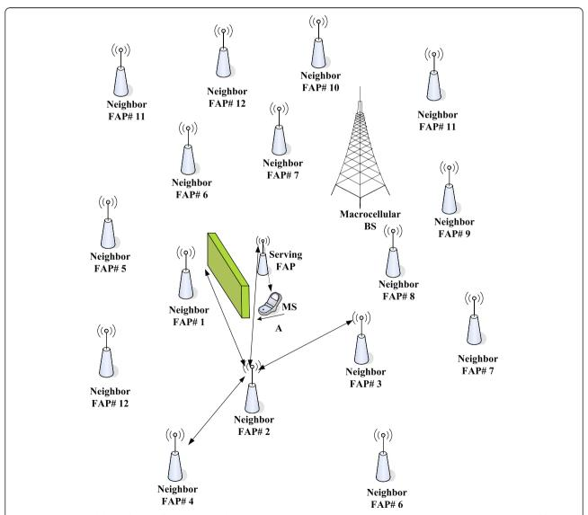
Figure 3 Scenario of dense femtocellular network deployment where several hidden FAPs and other FAPs are situated as neighbor femtocells.
