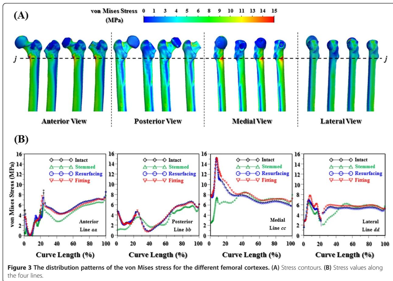
**Figure 3** The distribution patterns of the von Mises stress for the different femoral cortices. (A) Stress contours. (B) Stress values along the four lines.
