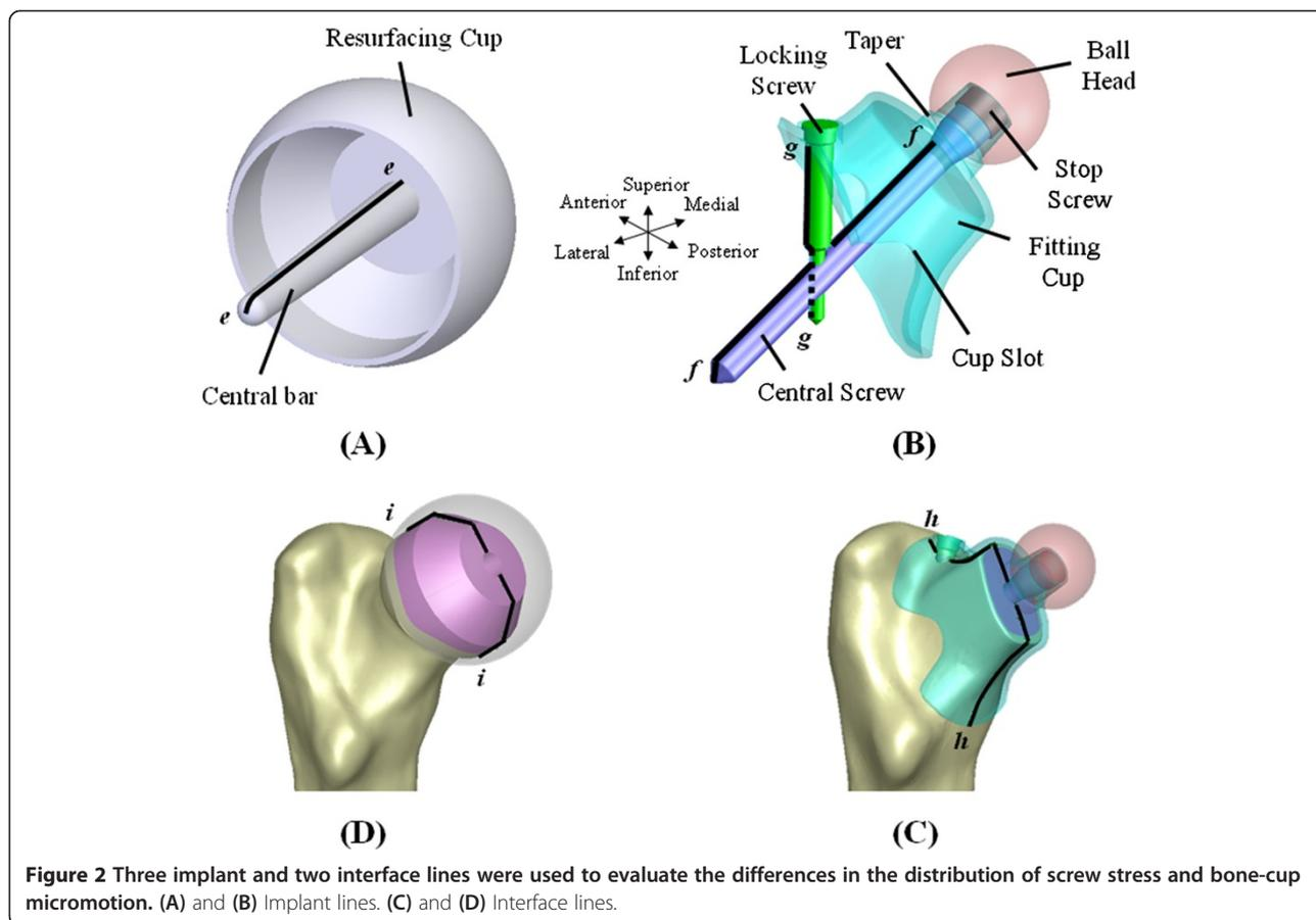
**Figure 2** Three implant and two interface lines were used to evaluate the differences in the distribution of screw stress and bone-cup micromotion. (A) and (B) Implant lines. (C) and (D) Interface lines.
