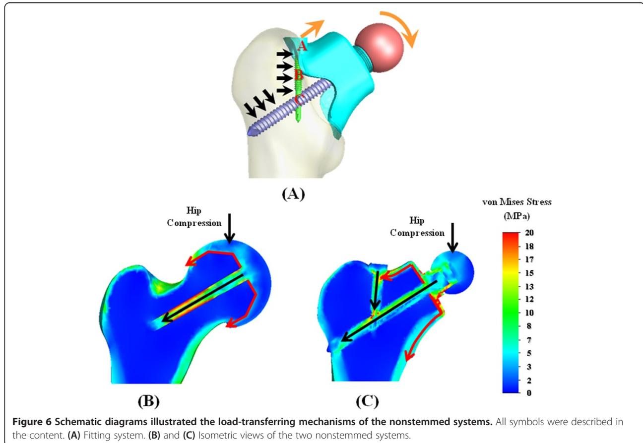
cup is superimposed over the reamed cancellous bone (Figure 2C and D). Consequently, the differences in contact situation, locking mechanism, and bone strength contribute to greater stability of the fitting than the resurfacing system. As in the resurfacing system, however, the downward movement of the fitting cup inevitably leads to interfacial micromotion at the distal portion of line *hh* (Figure 4B).
