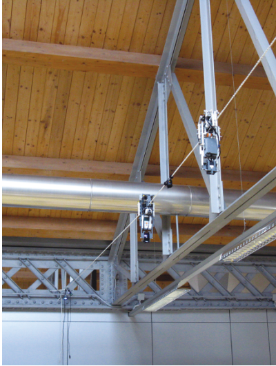
FIGURE 12: Photograph of the test bed, showing the two trams approaching the center node (SN2), with SN4 and DL visible in the background.
