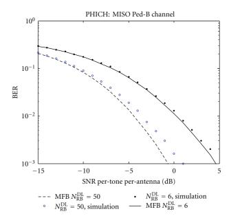
FIGURE 8: PHICH performance in Ped-B channel.
