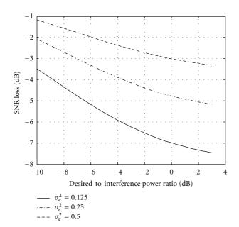
FIGURE 4: Effect of channel estimation error in PHICH.
