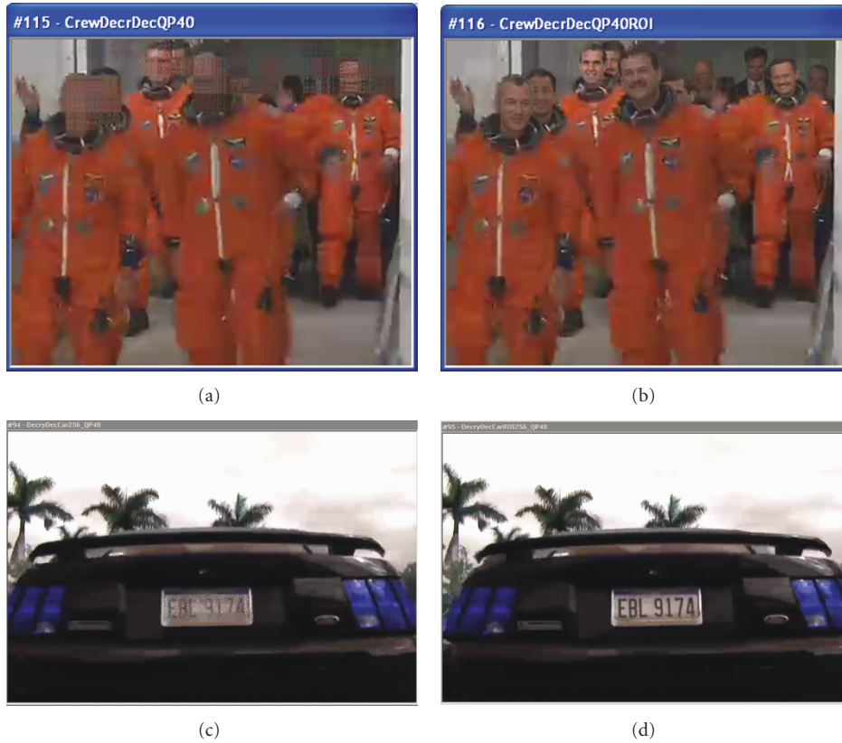
FIGURE 7: (a), (c) Decoded and decrypted H.264 video with QP of 40; (b), (d) decoded and decrypted H.264 video with QP of 40 and with ROI QP fixed to 26.
