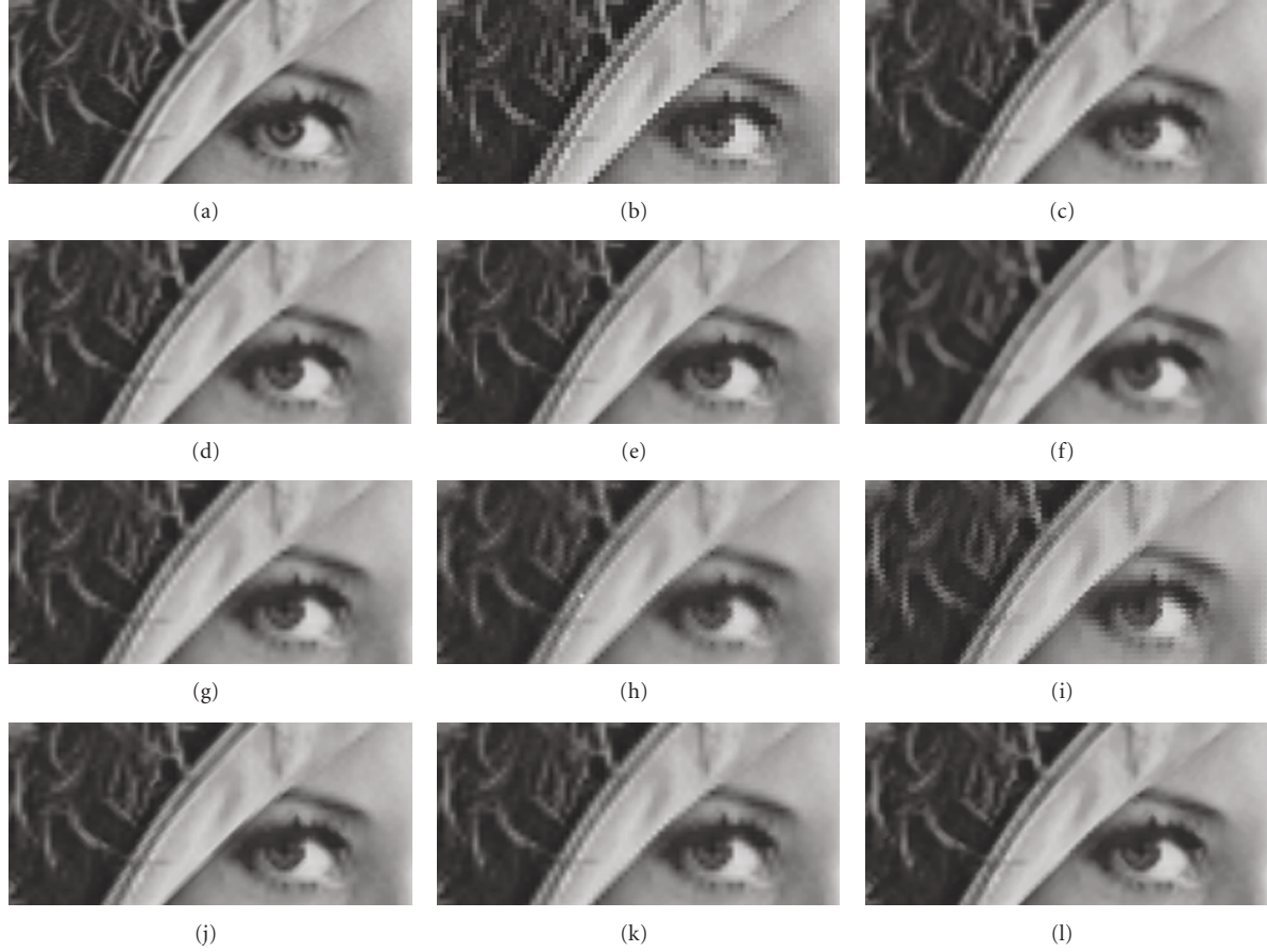
FIGURE 9: Close-up part of (a) original Lena image and its reproduced version interpolated by (b) Nearest Neighbor, (c) Bilinear, (d) WaDi-Bil, (e) Adaptive-Bil, (f) CFLS, (g) ESIF, (h) EDI, (i) EOA, (j) LAZA, and (k) SAI and (l) the proposed method.
