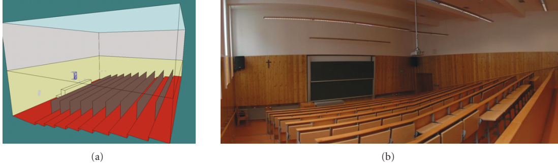
FIGURE 5: In the left figure, the 3D model of the simulated acoustic environment of the auditorium is depicted. The right figure is the photo of the modeled auditorium.
