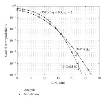
FIGURE 2: Symbol error probability of 8-PSK  $\mathfrak{G}_2$  and 16-QAM  $\mathfrak{G}_4$  OSTBCs (3 bits/s/Hz) versus  $E_s/N_0$  in MIMO Nakagami-q fading channels. q = 0.3 and  $n_r = 2$ .
