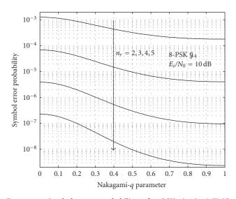
FIGURE 4: Symbol error probability of 8-PSK  $g_4$  in MIMO Nakagami-*q* fading channels as a function of the Nakagami-*q* parameter.  $n_r = 2, 3, 4, 5$  and  $E_s/N_0 = 10$  dB.
