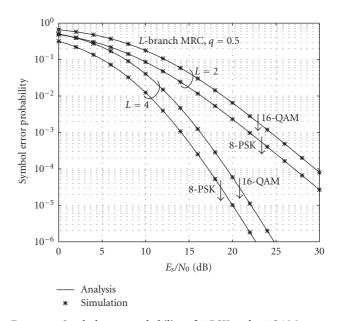
FIGURE 1: Symbol error probability of 8-PSK and 16-QAM versus  $E_s/N_0$  for *L*-branch MRC in SIMO Nakagami-*q* fading channels. q = 0.5, L = 2 and 4.
