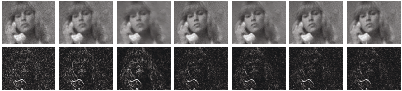
(g-2) Corrupted LR image (Poisson) (PSNR = 27.9071 dB) (g-3) L1 SRR image with Lap reg. (PSNR = 28.9197 dB) ( \beta = 1, \lambda = 1 ) (g-4) L1 SRR image with BTV reg. (PSNR = 29.1201 dB) ( \beta = 0.5, \lambda = 0.4, P = 2, \alpha = 0.7 ) (g-5) L2 SRR image with Lap reg. (PSNR = 30.7634 dB) ( \beta = 0.5, \lambda = 1 ) (g-6) L2 SRR image with BTV reg. (PSNR = 30.8631 dB) ( \beta = 0.5, \lambda = 0.5, P = 1, \alpha = 0.7 ) (g-7) Lor. SRR image with Lap reg. (PSNR = 30.6934 dB) ( \beta = 0.5, \lambda = 1, T = 9 ) (g-8) Lor. SRR image with Lor.-Lap reg. (PSNR = 30.8829 dB) ( \beta = 0.5, \lambda = 1, T = 5, T_g = 9 )
