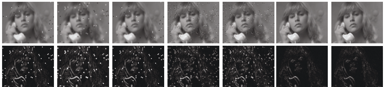
(i-2) (S&P:D = 0.01) Corrupted LR image (PSNR = 26.4446 dB) (i-3) L1 SRR image with Lap reg. (PSNR = 27.7593 dB) ( \beta = 1, \lambda = 1 ) (i-4) L1 SRR image with BTV reg. (PSNR = 26.4446 dB) ( \beta = 1, \lambda = 0.5, P = 1, \alpha = 0.7 ) (i-5) L2 SRR image with Lap reg. (PSNR = 29.8395 dB) ( \beta = 0.5, \lambda = 1 ) (i-6) L2 SRR image with BTV reg. (PSNR = 28.0337 dB) ( \beta = 0.5, \lambda = 0.4, P = 1, \alpha = 0.7 ) (i-7) Lor. SRR image with Lap reg. (PSNR = 34.7194 dB) ( \beta = 1, \lambda = 0.25, T = 5 ) (i-8) Lor. SRR image with Lor.-Lap reg. (PSNR = 34.7783 dB) ( \beta = 1, \lambda = 0.25, T = 9, T_g = 3 )
