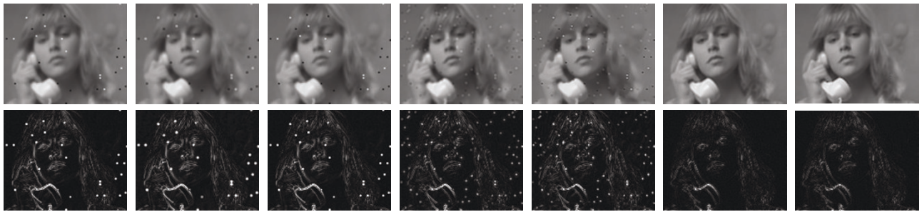
(h-2) Corrupted LR image (S&P:D = 0.005) (PSNR = 29.0649 dB) (h-3) L1 SRR image with Lap reg. (PSNR = 29.5041 dB) ( \beta = 1, \lambda = 1 ) (h-4) L1 SRR image with BTV reg. (PSNR = 29.0649 dB) ( \beta = 1, \lambda = 0.5, P = 2, \alpha = 0.7 ) (h-5) L2 SRR image with Lap reg. (PSNR = 31.5021 dB) ( \beta = 0.5, \lambda = 1 ) (h-6) L2 SRR image with BTV reg. (PSNR = 30.4617 dB) ( \beta = 0.5, \lambda = 0.4, P = 1, \alpha = 0.7 ) (h-7) Lor. SRR image with Lap reg. (PSNR = 34.7155 dB) ( \beta = 1, \lambda = 0.25, T = 9 ) (h-8) Lor. SRR image with Lor.-Lap reg. (PSNR = 34.7921 dB) ( \beta = 1, \lambda = 0.25, T = 9, T_g = 3 )
