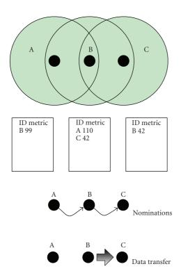
FIGURE 9: Hidden-station example. Radio range is shown by the shaded circles. Node B can communicate with A and C while A and C cannot communicate. After neighbor discovery, the neighbor tables are filled as shown. A nominates B, B nominates C, and C nominates itself in the election. B ignores A's nomination and A times out. C accepts B's nomination. B then sends data to C, and A does not transmit any data during this network wakeup.
