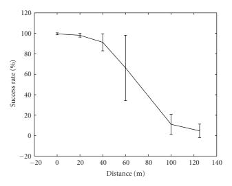
FIGURE 10: CSN-to-CSN range test. This test was conducted across a field with waist-high vegetation. Both collars were elevated 2 m. Bars indicate one standard deviation.
