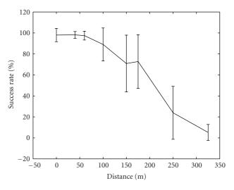
FIGURE 11: CSN-to-SRN station range test. This test was conducted across a field of waist-high vegetation. The base station was equipped with a high-gain  $(12\,dBi)$  directional antenna. Both nodes were elevated 2 m. Bars indicate one standard deviation.
