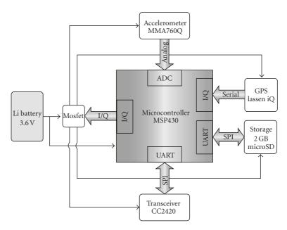
FIGURE 2: Top level block diagram of the CARNIVORE hardware. Black arrows indicate power connections. Thick shaded arrows indicate control and data connections.
