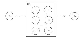
FIGURE 3: End-to-end message delivery under dominating-setbased routing.
