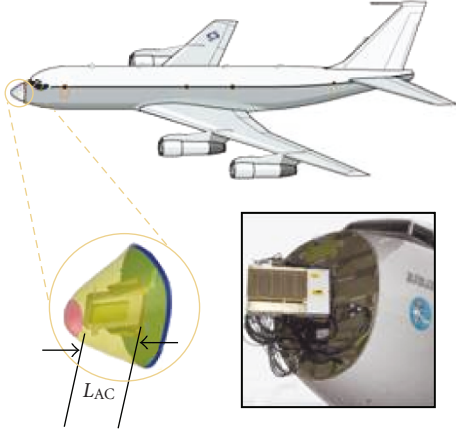
FIGURE 3: The 8-Channel X-band LiMIT system, mounted on a Boeing 707. L_{AC} \approx 18'' (source: Lincoln Laboratory briefing, December 2004).
