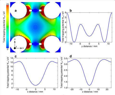
**Fig. 3 a** Total trapping potential around the trap center for Ca<sup>+</sup> ions. The trap radio frequency is  $\Omega=2\pi\times3.275$  MHz with 800 V<sub>pp</sub> amplitude and the DC endcap potential is 5 V. The extraction electrodes are grounded. **b** 1D cut through the potential along the y axis. **c** 1D cut through the potential along the x axis. **d** 1D cut through the potential along the z axis
