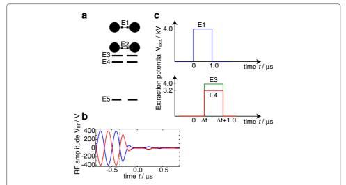
**Fig. 6 a** Schematic representation of the ion trap with the extraction and acceleration electrodes labeled E1-E5. **b** Oscilloscope traces of both radio frequency phases at the time when the RF generator is switched off. The dashed line indicates the switch-off time. **c** High voltage pulse sequence to eject ions from the trap and accelerate them. The optimal value for  $\Delta t$  is dependent on the ion mass-to-charge ratio. See text for details
