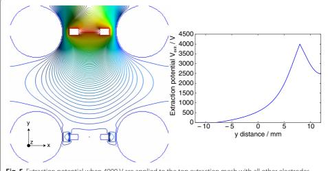
$\textbf{Fig. 5} \ \ \text{Extraction potential when 4000 V are applied to the top extraction mesh with all other electrodes grounded}$
