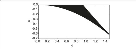
**Fig. 2** Stability diagram generated from MD simulations of a single Ca<sup>+</sup> ion at room temperature inside the ion trap. Trap frequency  $\Omega = 2\pi \times 3.275$  MHz
