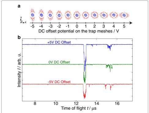
**Fig. 4 a** Molecular dynamics simulations of 100 Ca<sup>+</sup> (*blue*) and 100 ions of mass 80 u (*red*) at different DC offset potentials applied to the extraction meshes. **b** Time-of-flight traces of Coulomb crystals consisting of Ca<sup>+</sup>, CaO<sup>+</sup> and CaOH<sup>+</sup> ions at different DC offset potentials applied to the extraction meshes prior to the ion extraction. Each trace is the average of 5 measurements
