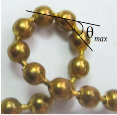
Fig. 2. \theta_{\max} is the maximum angle between the two consecutive links and determines the rigidity of the chain. \theta_{\max} and l_p of the chain used in our experiments are 45^\circ and 21 mm respectively. The minimum number of beads required to form a ring is roughly the same as the persistence length of the chain.
