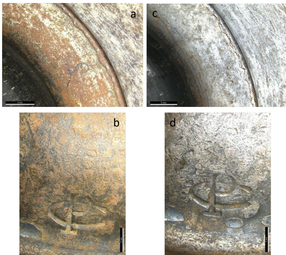
Fig. 10 Digital microscope images of details from the candleholder before a, b and after c, d cleaning. Scale bar indicates 5 mm
