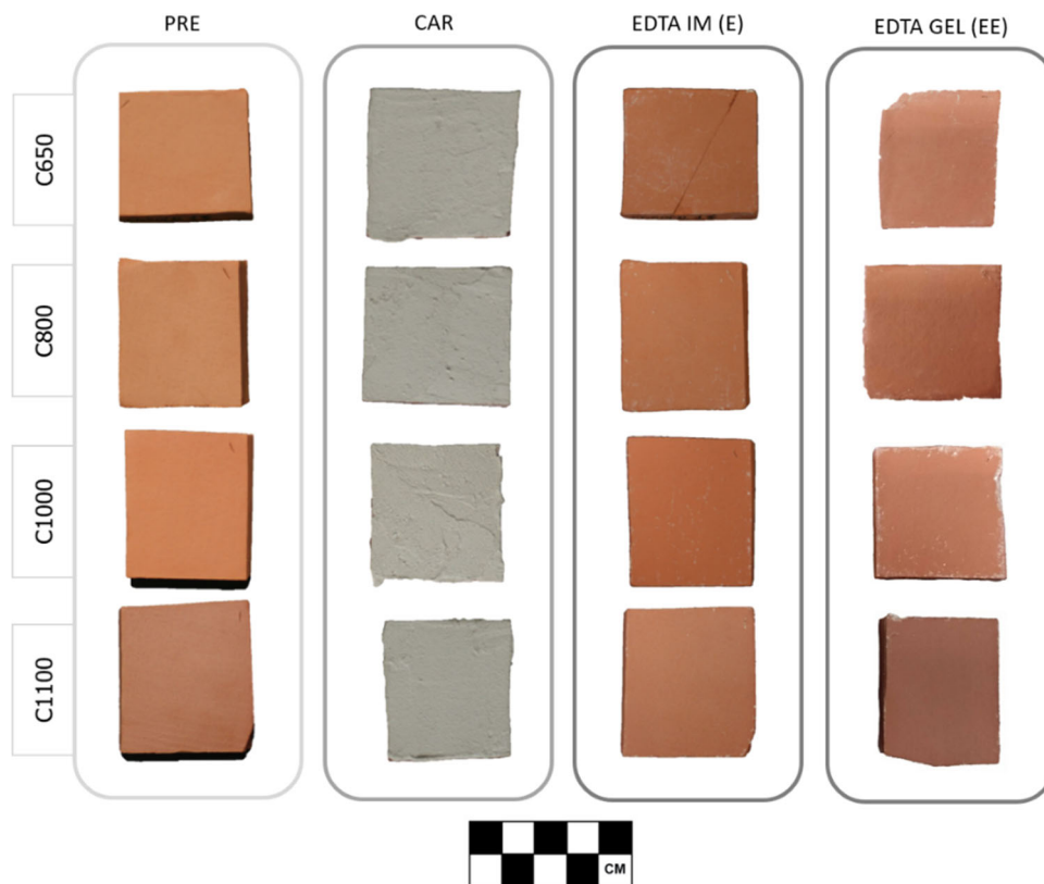
Fig. 3 The appearance of the ceramic specimens before and after the carbonation process (PRE and CAR, respectively), and the treated specimens with the solution of \text{Na}_4\text{EDTA} by immersion (E) and thickened with Vanzan® NF-C (EE)
