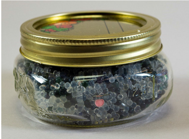
Fig. 1 A 250 ml Mason Ball jar used as an oxygen consumption monitoring vessel
