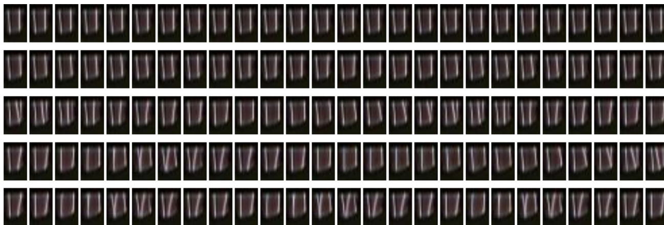
Fig. 8 Image sequences of the transition between stationary and locked mode with three filaments. The gas flows through the capillary from top to bottom. The first row shows the stationary mode. The filaments do not move. In the second row, the right filament moves alternating to left and right. The movement starts at and is dominated by the point at the top electrode. The third row shows alternating movements of all filaments first to the right and then to the left. The last row finally shows the locked mode. All filaments move in one direction around the capillary. The images in one row have a time gap of 5 ms. The time between the rows is larger
