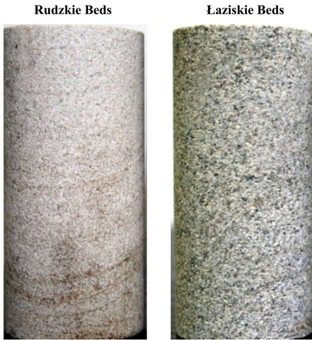
Fig. 1 Exemplary samples prepared for uniaxial compression tests: on the left the very fine-grained sandstone—Rudzkie Beds; on the right: the medium-grain sandstone—Łaziskie Beds
