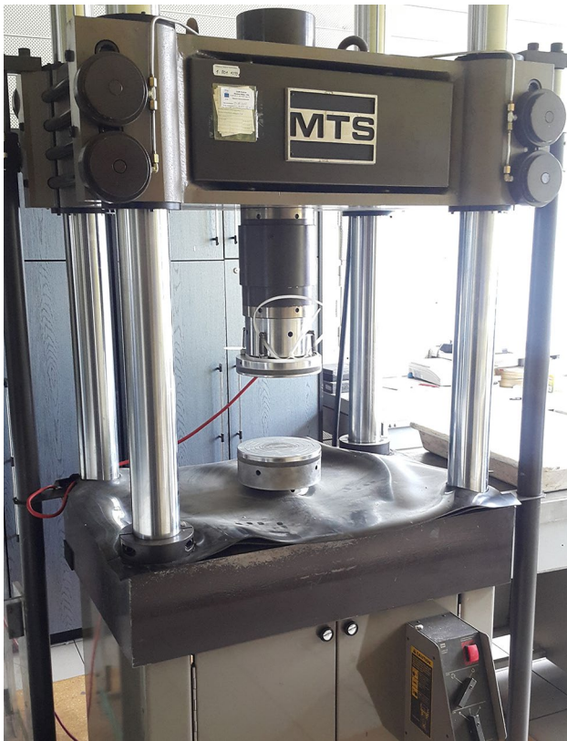
Fig. 3 Servo-controlled testing machine MTS-810 used for meso-scale investigation
