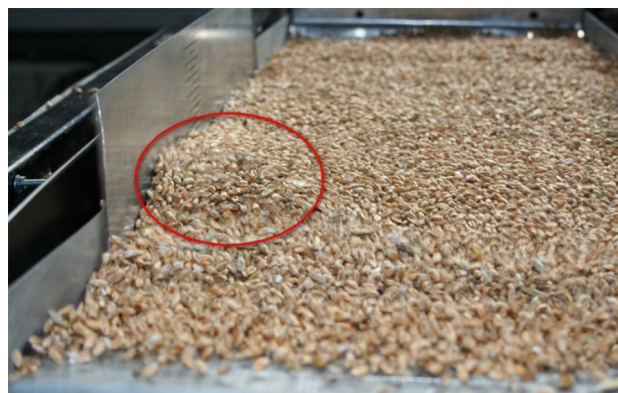
Fig. 3 Behavior of moving grain mass affected by air stream (red circle: area of the bubble created by initial fluidization)
