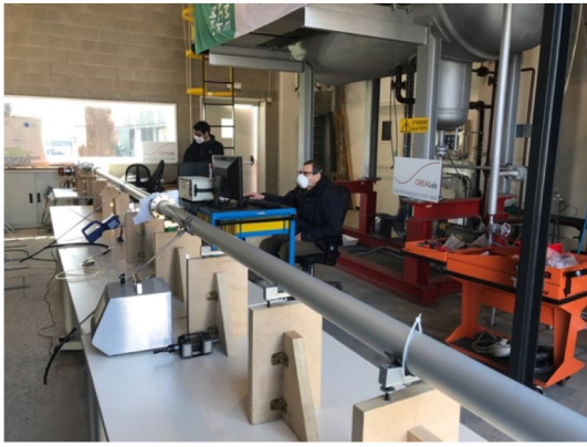
Fig. 2 One of the testing facilities set up by Politecnico di Milano for the certification of surgical masks and PPE
