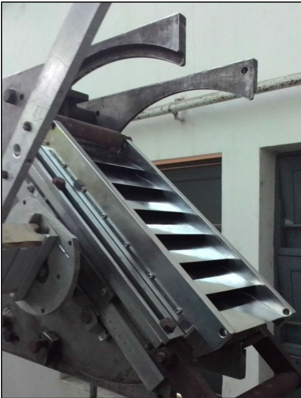
Fig. 7 Cascade installed in the tunnel
