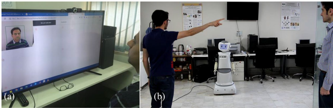
Fig. 6 a Calibration of the Attention's formulation: a participant sitting in front of the screen and performing the calibration process in WebGazer, before the start of the gaze pattern recording. b Evaluation of the GCS: a volunteer interacting with the robot and one of the researchers to assess the performance of the robot
