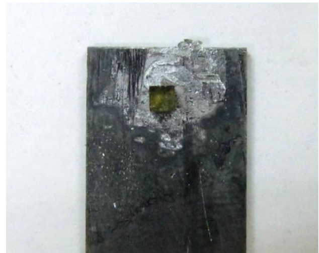
Fig. 3 Joint specimen comprising diamond soldered to a Mo plate
