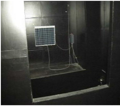
Fig. 1 PV module placed in QuickSun 700A large area solar simulator chamber for testing purpose
