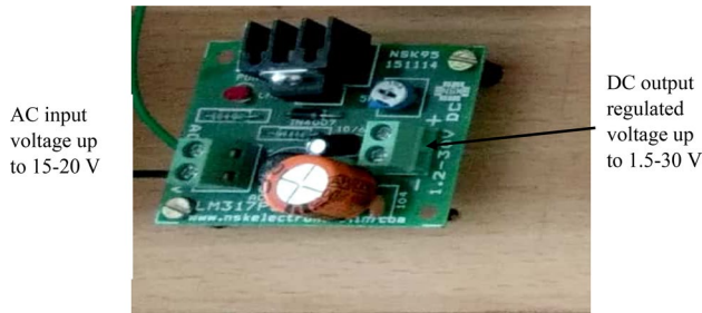
Fig. 8 Adjustable voltage regulator
