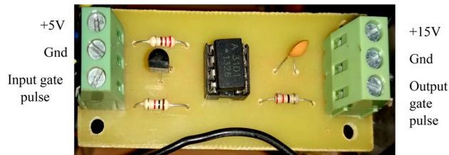
Fig. 9 Gate driver circuit
