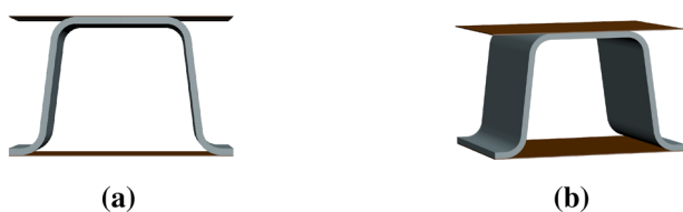
Fig. 1 The UHSS sandwich concept is evaluated by subjecting a hat-profile geometry to crushing. A frontal view is presented in a and a perspective view is presented in b . The barrier on top crushes down on the hat profile, while the flange edges are clamped and the support below is fully fixed
