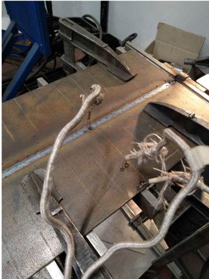
Fig. 2 Welded joint with all of the thermocouples attached
