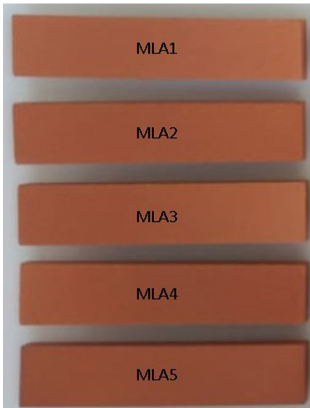
Fig. 3 Roofing tile pieces sintered at 1100 °C
