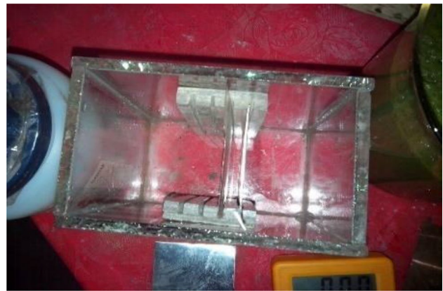
Fig. 3 Experimental set-up; plastic separator and holder inside the rectangular glass box holding the electrodes
