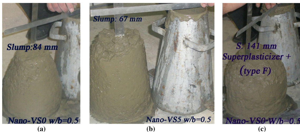
Fig. 4 Slump test photos of some fresh concrete mixes (a and b concrete mixes made with no superplasticizer and c with superplasticizer added)
