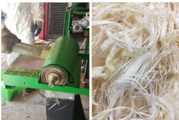
Fig. 2 Device for fibre extraction (left) and obtained fibres (right)
