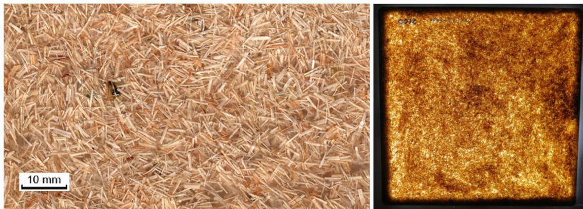
Fig. 4 Composites obtained with untreated Agave americana L. fibres at 30% (left). Plate with 10% of fibre, showing fibres distribution in the matrix (right)
