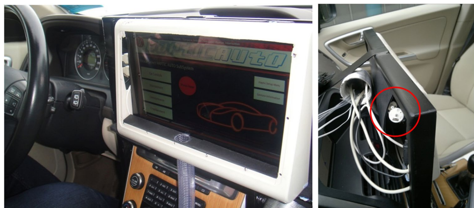
Fig. 4 Custom vibrotactile actuation prototype with specifically designed rear mounted actuator shaft for the ExoPC slate tablet
