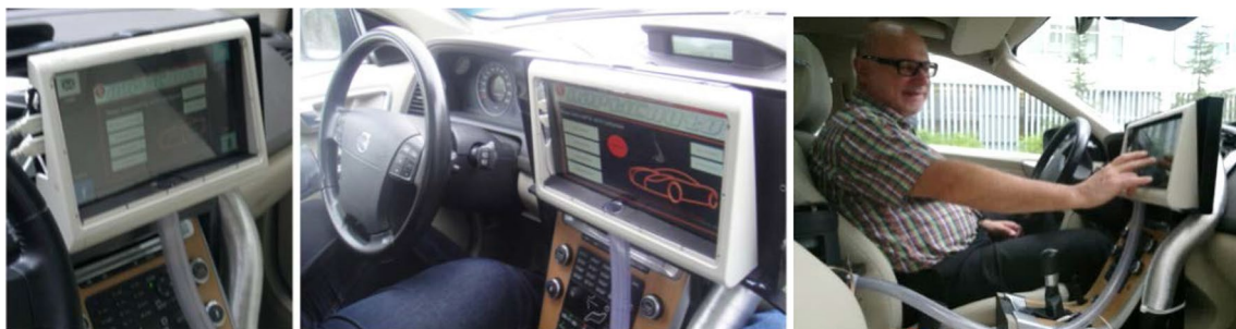
Fig. 1 The PSW prototype provides pneumatic feedback from the bottom of the touchscreen
