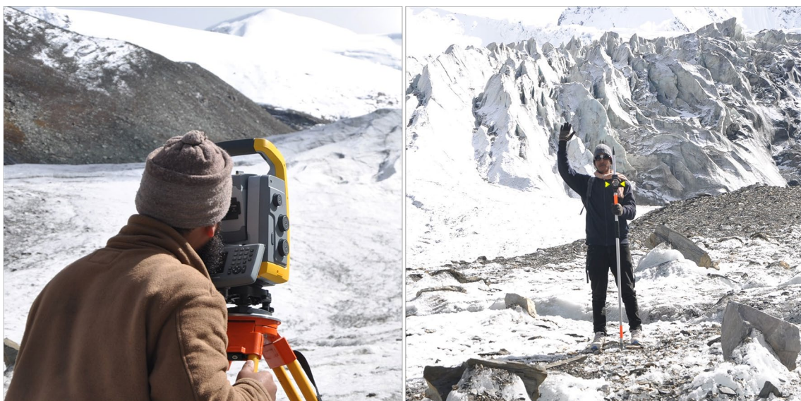
Fig. 2 Operation of the Trimble Electronic Total Station (ETS) in the field
