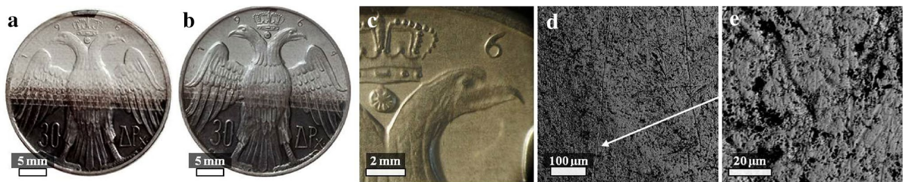
Fig. 8 Coin 30_DR: a optical image after the laser irradiation. b Optical image after wiping the solid silver from the coin's surface. c OM image of the cleaned area. d SEM image on backscattered
