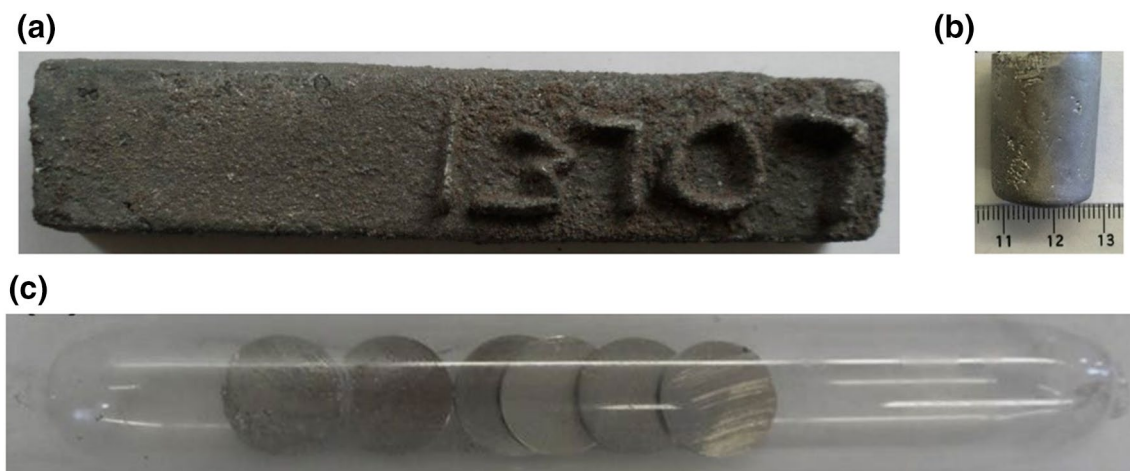
Fig. 1 a Keel bar selected for the experiment. b Example of a recast sample solidified at a controlled rate. c Typical encapsulated samples for controlled cooling from the homogenization temperature
