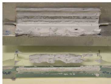
Fig. 10 Typical failure patterns from the experimental tests on linear adhesive joints under tensile loading
