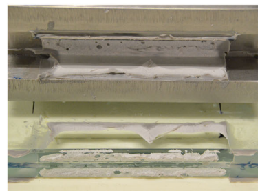
Fig. 10 Typical failure patterns from the experimental tests on linear adhesive joints under tensile loading
