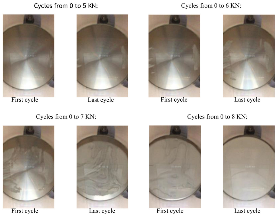
Fig. 16 Whitening effect propagation under loading cycles
