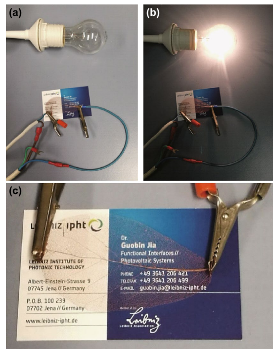
Fig. 4 Demonstration of high current density transport capability. a The 30 min as-plated MLLV is connected between the cables. b A bulb (40 W and 230 V) shines if the switch is tuned on. c Photograph taken as the applied current of 1 A was passing through the Cu-plated vein
