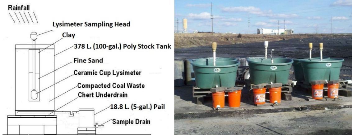
Fig. 3 Field kinetic test columns (left); photograph of field test site (right)
