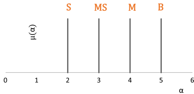
Fig. 6 The membership functions regarding \alpha in the fuzzy-based system
