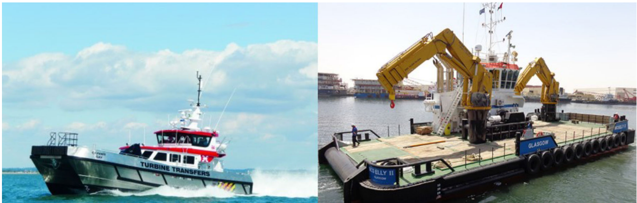
Fig. 10 Representation of a CTV and a multicat vessels
