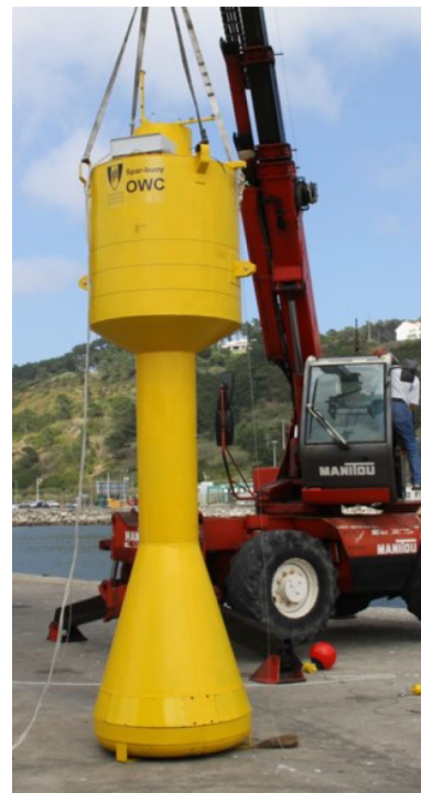
Fig. 3 Spar–Buoy prototype scale 1/16th
